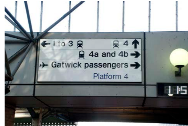
Overstating directions, conflicting information (saying platform 4 is ahead and indicating that platform 4 is here), weak sense of place (platform 4 is the lightest typography on the sign, it doesn't state or confirm that a traveler is where he needs to be).
